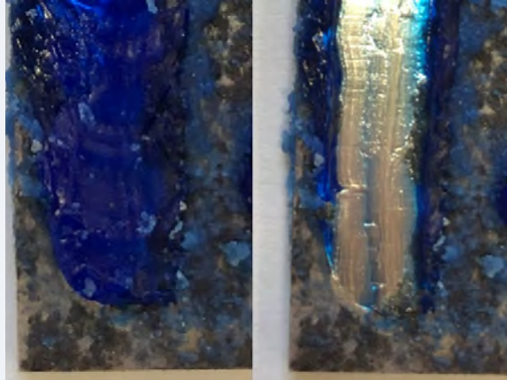
Protection against corrosive infiltration – after 6 weeks of PV 1209 in the open component, left before and right after removal of the permanently plastic sealant
