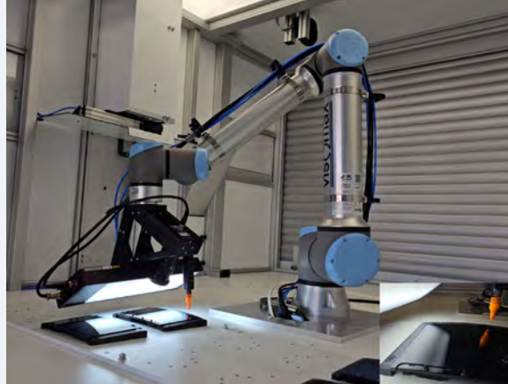
Line scan camera with special lighting technology on a 6-axis robot
