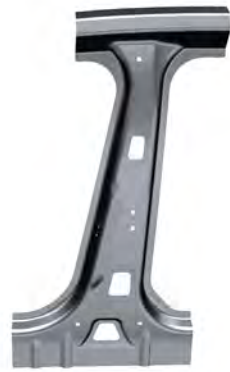
B-pillar made of Silicon-boron steel grade "SIBORA"
