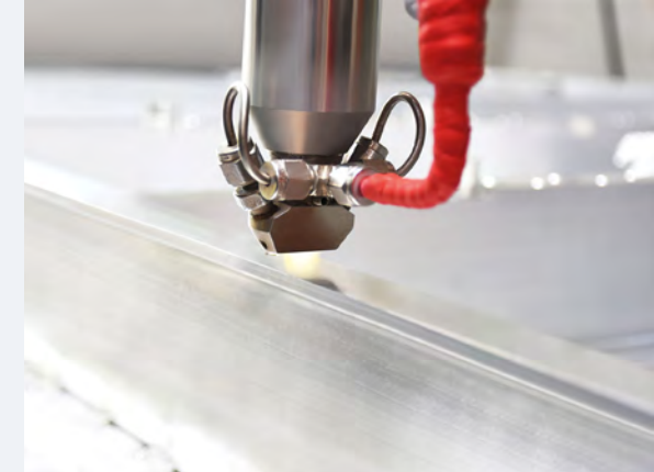
Plasma coating of a battery housing
