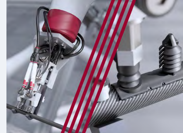
Automated Gluing Locator
